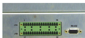
Straight forward rear panel I/O connections
