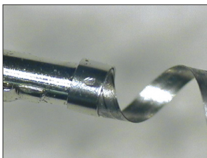
0.002 in thick platinum strip to platinum tube
